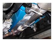
**2.** Install head pipe #A onto your existing stock front pipe and attach with hardware kit #F. DO NOT TIGHTEN. Insert welded hangers into rubber grommets.
